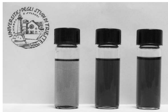
Fig. 1 Pristine SWNHs in chloroform (left) and nanohorns 1 in chloroform (middle) and in DMF (right).
